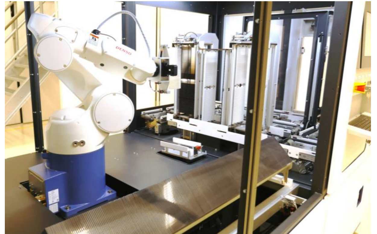
SiC boat 1000 wafers loading and unloading within 15 minutes
